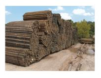
treated wet might look protected at first glance, any crack the post incurs will be an open invitation for environmental moisture, leading to fungal decay and insect infestations.
