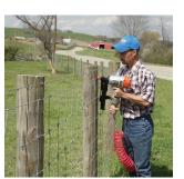
Anyone who has ever built a fence knows that the most time-consuming and painful part is hammering staples in by hand. Now there is a much better alternative. The Stock-ade ST-400 pneumatic stapler is ideal for farm fencing. It is durable and very powerful and will drive fence staples into the hardest posts you can find. It shoots a 1 3/4" or 2", 9 gauge, barbed staple and features a sequential trigger system, a depth of
